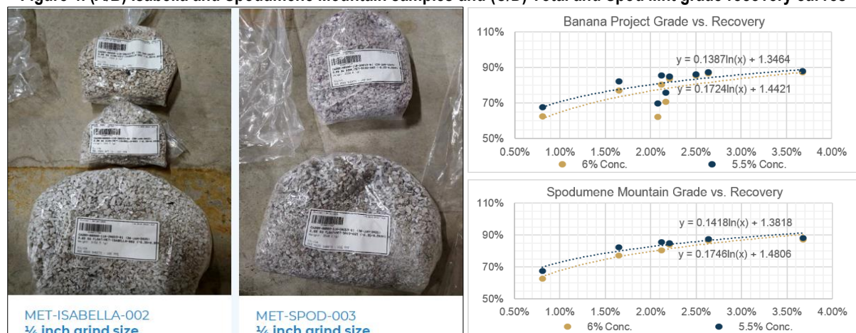
Figure 4. (A/B) Isabella and Spodumene Mountain samples and (C/D) Total and Spod Mnt grade recovery curves
