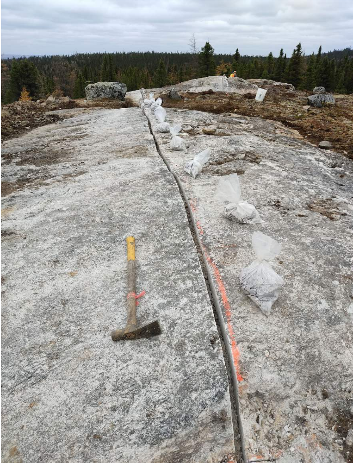
Channel sampling at Spodumene Mountain. A total of 66 1-metre-long samples were taken from the three channels in the Phase 2 exploration program
